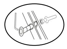
Repeat Step2 ,attach BasketTop(A) to Basket Middle(B) ,using Screw(F) and Nut (G) with Allen Key (H) and Spanner(I). **DO NOT OVERTIGHTEN.**
