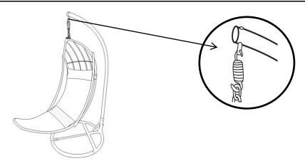
Lift the Chair-Basket and hook-loop the Iron Chain into the hook on the Iron Stand(K) as shown above.
