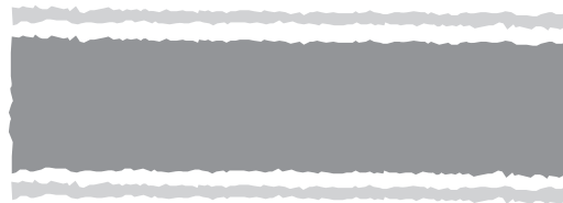
POOR SPRAY PATTERN (TAILING)
