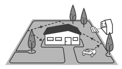
The mower moves randomly within its working area, as defined by the perimeter wire. This kind of random movement provides the perfect cut and ensures complete coverage of your lawn.
