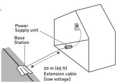
Connect the DC cable from the Power Supply unit to the 20 m (65 ft) extension cable.
