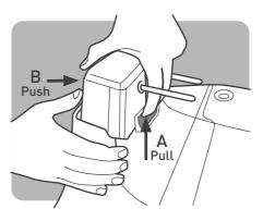
Feed both the Perimeter Wire (A) and the extension cable (B) through the slot in the rear side of the Base Station.
