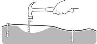
Hammer the extension cable into the ground so it's not a tripping hazard.
