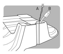
Attach the Perimeter Wire connector to point A on the Base Station's head. Attach the 20 m (65 ft) extension cable to point B on the Base Station's head.
