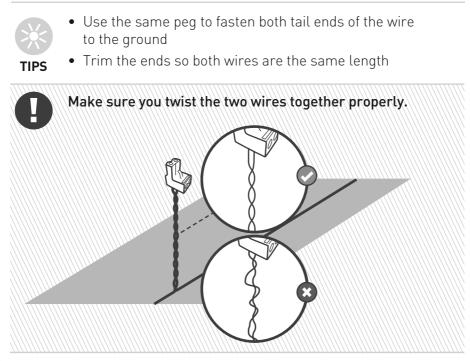
Strip back 5 mm (0.2 in) of insulation from the wire ends, insert the twisted wire into the connector and secure it using a small flat screwdriver.
