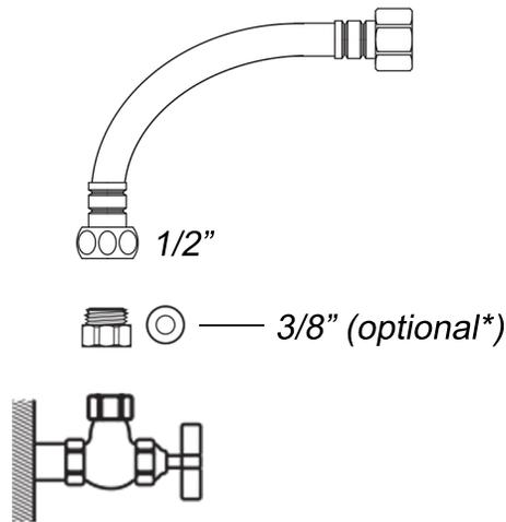
*\*You may need to use the included conversion nut to fit your water shutoff valve. Simply screw the conversion nut into the 1/2" side of the hose before connecting it to your water shutoff valve.*
