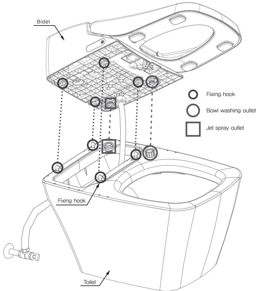
*\*Do not use excessive force when attaching the bidet seat to the toilet base.*
