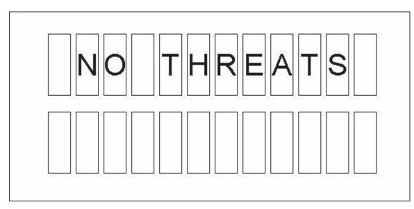
This message indicates that Tornado Alert<sup>™</sup> is functioning normally and no severe weather conditions exist. If activity is detected, one of the following messages, ranked from least to most significant, will be displayed:
