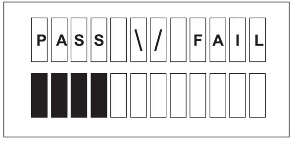
In order to pass this test, no activity should be detected for 20 seconds. If excessive activity is detected, more bars will be darkened to the right, the LED light will turn red and the test will restart. Find a
