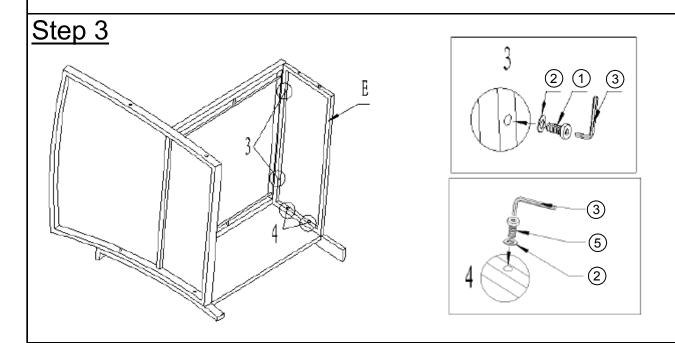
Place Front Panel(E) between Seat(D) and Right Armrest(C). Attach Front Panel (E) to Seat(D) using Hardware(125) with Allen Key(3) as shown in Picture 3 and Picture 4. **Do not fully tighten at this stage.**
