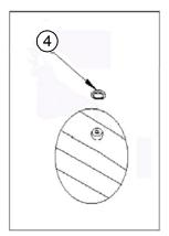
Fully tighten all bolts at all joints, then cover the four Backrest Bolts with Nut Cap ( 4 ).
