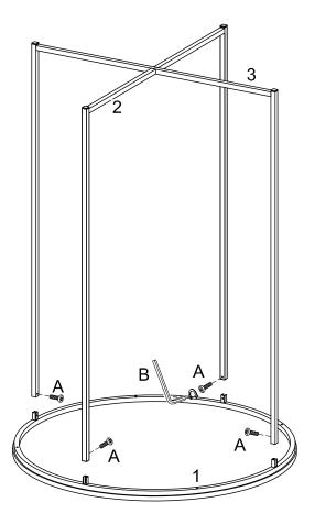
Use wrench (B), to secure legs (2,3) to table top (1) with bolts (A).
