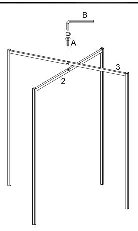
Use wrench (B), to secure legs (2,3) with bolt (A).
