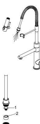
Pull the hose assembly out of the spout and remove the spray head by unscrewing it from the hose in a counterclockwise direction. Be sure to hold the end of the hose down into the sink and turn the faucet on to the warm position where it mixes hot and cold water.
