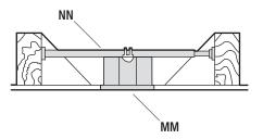
To hang your fan where there is an existing fixture but no ceiling joist, you may need an installation hanger bar (NN) (not included) as shown above.
