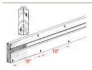
**(G)** Drill 3/32" holes in base moulding and inside corner block.
