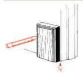
(I) Position plinth block at base of door jamb (see #5 in illustration at top of page). Set plinth block approximately 1/8" back from jamb. Mark wall with pencil line on left side of plinth.
