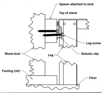
For other types of wall: use seismic/mounting clips (included) with appropriate anchors (not included).
