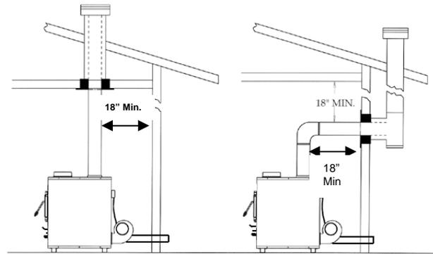
**Figure 2 – Installation into a HT Pipe Flue System**
