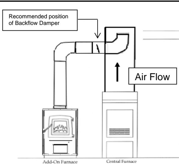
**Figure 3 – Hot air outlet hook-up to ductwork**
