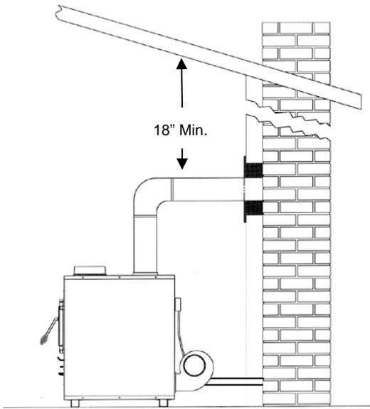
**Figure 1 – Installation into a Masonry Flue**
