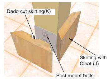
**24.** Locate all Post Skirting pieces. Position 2 post skirtings around the base of post as shown above. Use 1 Post Skirting with Cleat - 1 1/2" x 9" x 10" (Part J) and a Post Skirting with Dado Cut - 1 1/2" x 9" x 10" (Part K) initially. Cleat piece should be aligned opposite post mount hardware and dado piece aligned with post mount bolts (hardware).
