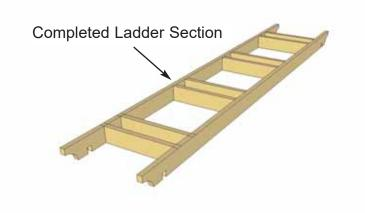
**13.** Complete all four Ladder Sections on the ground prior to moving to **Step 14.**
