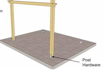
**4.** Secure Post to Post Hardware with appropriate hardware such as lag bolts or a sufficient number of screws.(Hardware Not Supplied)
