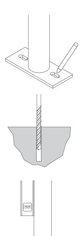
**1.** Place the rack in the desired location. Use a marker or pencil to outline the holes of the flange onto the base material.
