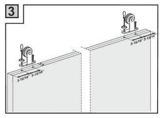
Drill holes in the top of the door 3-15/16" from the edge as pictured to accommodate the door rollers.
