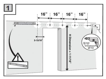
Find the centerline of the track. Using a level, mark a horizontal line twice the door width long. Mark the bracket screw locations into the wall blocking. Attach the wall portion of the brackets as shown.
