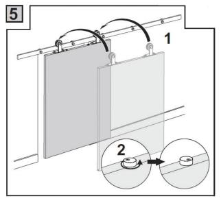
Attach the door to the rails making sure that the anti-jump disks are engaged to avoid a serious accident.
