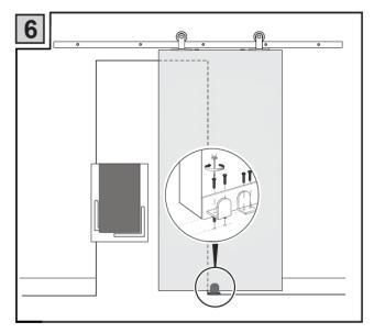
Plumb the door and mark the positions of the floor guides. Mount the floor guides to the floor.
