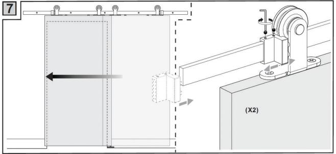
Adjust the door stops accordingly using the provided Allen key.
