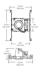
The 19000A-LED-ID features Ideal® connections that allows for quick, snap-in connection of NICOR® D-series LED downlights. Suitable for new construction in residential and commercial applications. IC rated. Suitable for direct contact with insulation.
