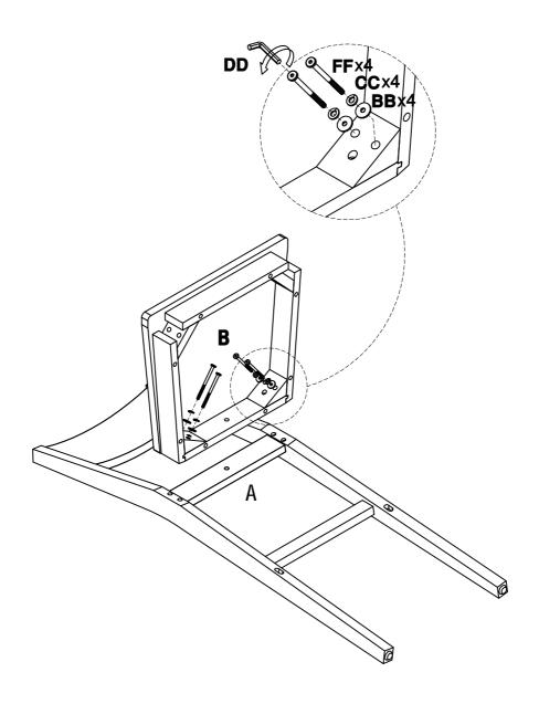
$2\,$  Use allen key (DD) to drive the screw(AA) with washers(CC&BB) as shown
