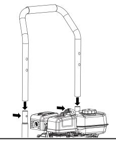
Install the storage panel and trigger handle
