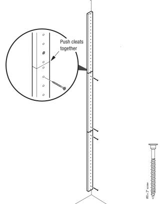
Corner shelves are supported by using either 48" or 72" vertical panels. Position one of the vertical panels on the floor as shown with front edge up. Attach bottom and middle corner shelf using #8 x 2" screws.
