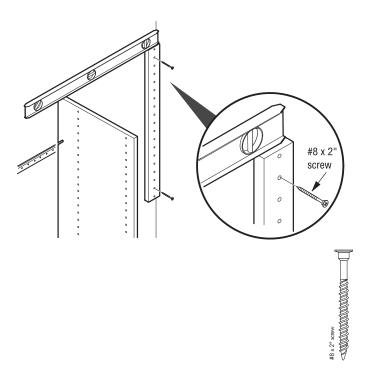
Remove vertical panel. Install 2nd and 3rd cleat to end of previously installed one with #8 x 2" screws. Two (2) cleats are supplied in one corner shelf kit. Two corner shelf kits are required for a 72" section.
