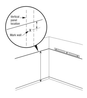
Locate studs. Tap the wall or use an electronic stud finder to locate studs. Mark wall 1/2" below horizontal line. Studs (2 x 4) are usually located on 16" centers measured from the left or right side.
