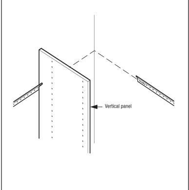
Position cleat in corner and level with vertical panel. Screw cleat to wall using two (2) #8 x 2" screws.
