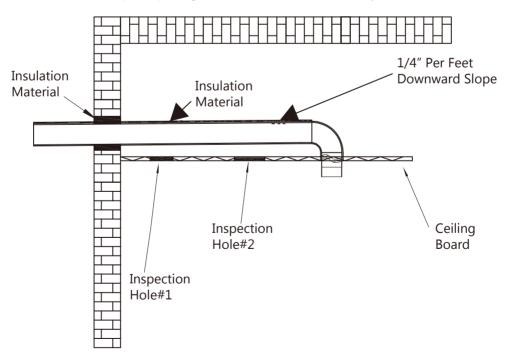
**NOTICE:** Vent pipes must be completely insulated with inflammable material when installed in alcoves, closets, and garages and must not touch any flammable material.
