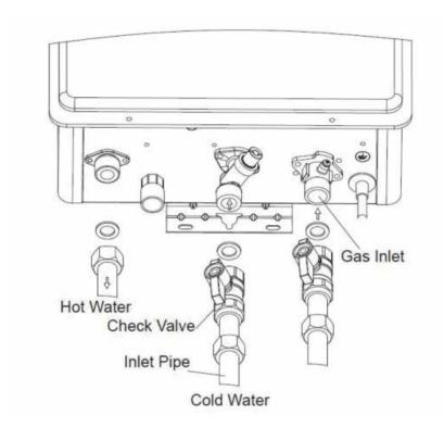
**NOTICE:** The hot and cold pipes should be insulated as shown help to provide additional freeze protection.
