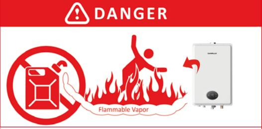
Vapors from flammable liquids will explode and catch fire causing death or severe burns
