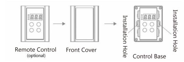
2. At installation site, mark and screw two holes with 0.24" with 1.2" depth. Insert 2 rubber screws into the holes. Place the remote control against the wall, align the holes of control with the holes in the wall, and fasten them with wood thread screws. (See illustration below)
