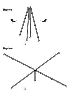
Insert connecting pipe of middle feet (C) to side tube (A) and (B) as shown.
