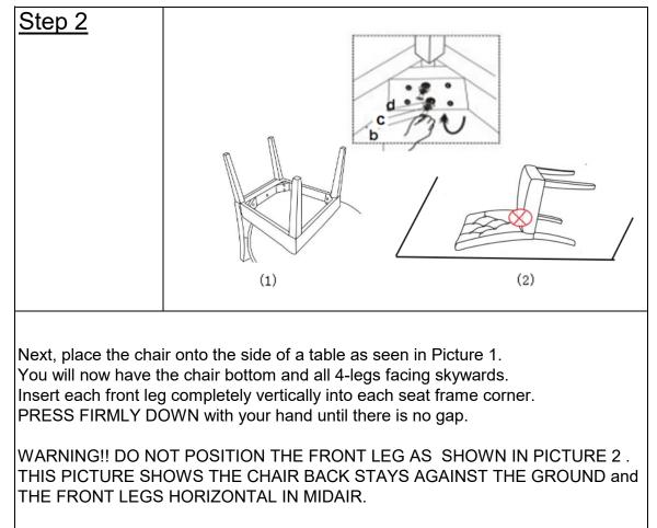
Now tighten the bottom bolt first, then the bolt on the top by using 4 Bolts (b) and 4 Spring Washers (c) and 4 Flat Washers (d). DO NOT tighten the top bolt first.
