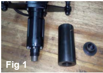
Fig. 1 ) Locate Pile Driver, Piling Socket & Inner Pile Head. Fig. 2 ) Attach Piling Socket by screwing it onto Pile Driver. Fig. 3 ) Make sure Piling Socket is secure.
