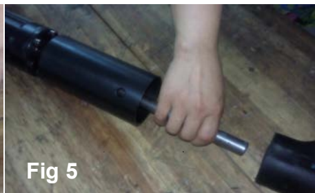
Fig. 4 ) Insert Inner Pile Head. Fig. 5 ) Insert Piling Socket Pin then rotate. Using a mallet, hammer into Piling Socket until secure. Fig. 6 ) Piling Socket is assembled.
