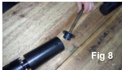
Fig. 7 ) To disassemble, remove Piling Socket Pin by using a mallet. Fig. 8 ) Remove Piling Socket Pin. Fig. 9 ) Unscrew Inner Pile Head.
