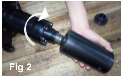
Fig. 1 ) Locate Pile Driver, Piling Socket & Inner Pile Head. Fig. 2 ) Attach Piling Socket by screwing it onto Pile Driver. Fig. 3 ) Make sure Piling Socket is secure.
