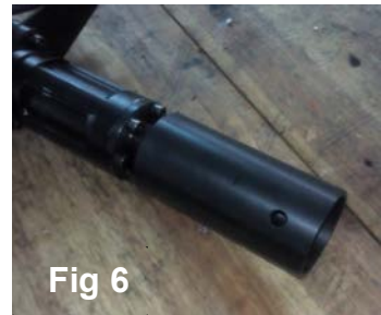
Fig. 4 ) Insert Inner Pile Head. Fig. 5 ) Insert Piling Socket Pin then rotate. Using a mallet, hammer into Piling Socket until secure. Fig. 6 ) Piling Socket is assembled.
