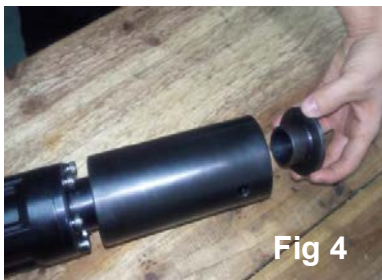
Fig. 4 ) Insert Inner Pile Head. Fig. 5 ) Insert Piling Socket Pin then rotate. Using a mallet, hammer into Piling Socket until secure. Fig. 6 ) Piling Socket is assembled.
