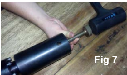
Fig. 7 ) To disassemble, remove Piling Socket Pin by using a mallet. Fig. 8 ) Remove Piling Socket Pin. Fig. 9 ) Unscrew Inner Pile Head.
