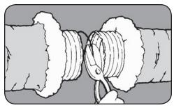
**Step 2:** Slide at least 1" [25 mm] of core over fitting and past the bead. Seal core to collar with at least 2 wraps of duct tape. Secure connection with clamp placed over the core and tape and past the bead.
