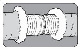
**Step 2:** Tape cores together with at least 2 wraps of duct tape. Secure connection with 2 clamps placed over the taped core ends and past the beads.
