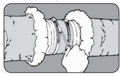
**Step 3:** Pull jacket and insulation back over cores. Tape jackets together with at least 2 wraps of duct tape.
