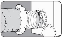
**Step 3:** Pull jacket and insulation back over core. Tape jacket with at least 2 wraps of duct tape. A clamp may be used in place of or in combination with the duct tape over the core and tape and past the bead.
