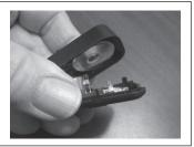
3. Replace battery top with the metal ring visible.
