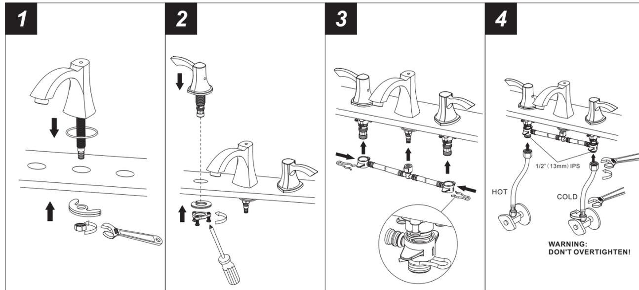
1. Position the body with o-ring in the installation surface as shown and secure it with gasket assembly and tighten the lock nut with adjustable wrench.
