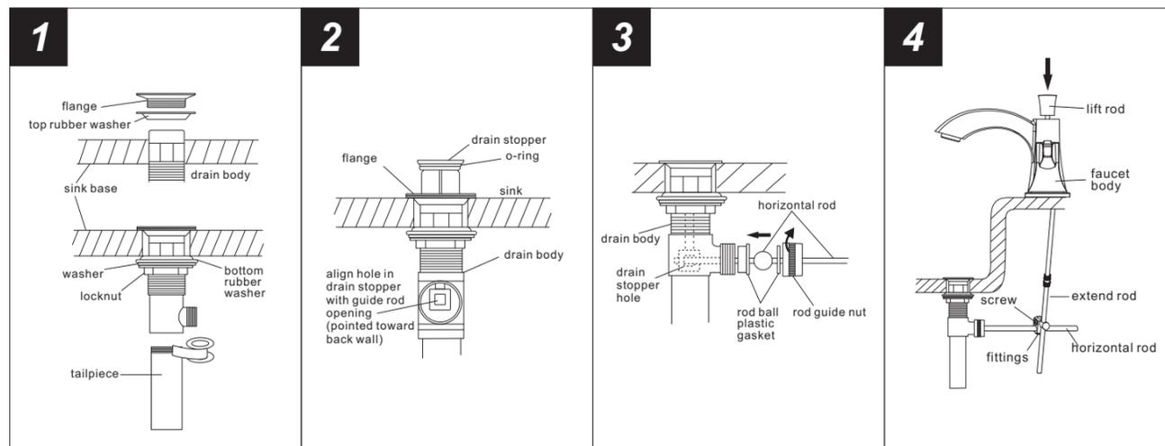
1. Remove pop-up drain stopper, and flange with top rubber washer for pop-up assembly. Insert drain body from underneath of sink drain hole. Replace flange and top rubber washer back to drain body. Tighten flange as far as possible. Remove and put silicone along bottom of. (Optional) Slide bottom rubber washer on drain body up against bottom of sink. Tighten washer and locknut firmly against base for tight seal. Remove tailpiece from drain body, add Teflon tape, replace tailpiece.
