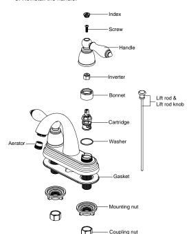
**Problem**: Faucet leaks around aerator or an improper flow pattern.
