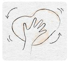
For solvent based adhesive, clean up surface with mineral spirits-dampened rag (do not use lacquer thinner). For low VOC adhesive, wipe off all excess adhesive on the surface with water dampened rag.
