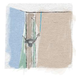
Put the first panel in place and bring to adjacent wall in the corner allowing 1/16"space. Make sure it is plumb and both left and right panel edges fall on solid stud backing.
