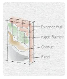
Installing paneling over existing true walls requires no preliminary preparation. Sanding high spots on the wall is generally about all you have to do.
