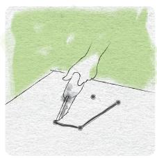
If measured floor-to-ceiling height is 8' or less, subtract 1/2" from this measurement to allow 1/4" expansion clearance on top and bottom. Transfer these measurements to panels for cutting.
