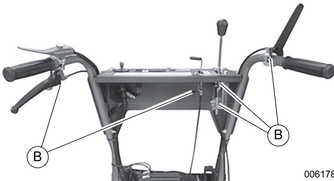
Figure 4-2. Cable Lubrication Locations
