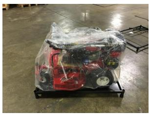
3. Using a Utility Knife carefully remove the plastic covering and a tie down straps as shown below.
