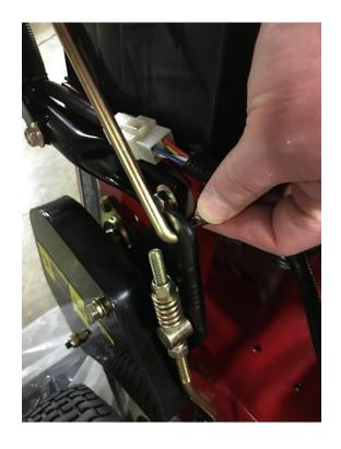
10. Locate drive lever rods and attach to left and right drive plates as shown above.
