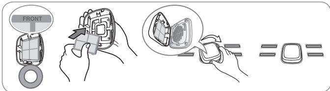
After changing the filter, push and hold the Air Filter button for three seconds to reset the filter sensor.
