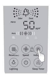
• In the example above, the PM1.0 density displays at 50 ug/m3 (a bad or orange level) and the dust particle size LED indicator for PM1.0 is lit. This indicates that the PM1.0 level is higher than the PM10 or PM2.5 levels. If all the PM density levels are normal/good and the air quality indicator light is orange/red, the level of odors is very high.
