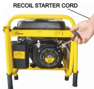
Figure 14- Pulling the start cord
