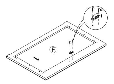
• ATTACH THE MAGNET (i) INTO BOTTOM OF THE FIXED PANEL (F) BY USING THE 5/8" L ROUND HEAD SCREW (d).
