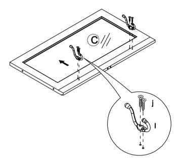
• ATTACH THE DOUBLE HOOK (I) TO THE TOP MIRROR FRAME (C) BY USING THE 1/2" L FLAT HEAD SCREW (j).
