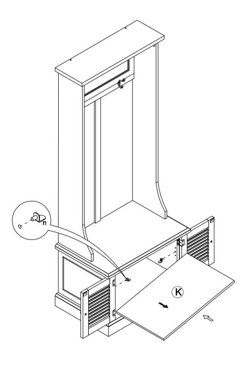
• PLACE THE SHELF PIN (n) IN DESIRED POSITION AND PLACE THE ADJUSTABLE SHELF (K) ABOVE THE SHELF PIN (n).
