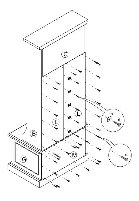
• TIGHTEN THE UPPER BACK PANEL (L) AND THE LOWER BACK PANEL (M) BY USING THE METAL PLATE (m) AND THE 5/8" L ROUND HEAD SCREW (d).
