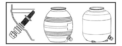
**2.** Press and turn the sand tank to mount it to the sand filter support with correct direction, drain plug on the outside (see below)
