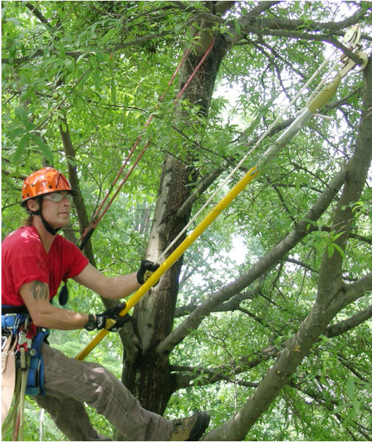
JA-14 Pruner Permanently Mounted on Pole
