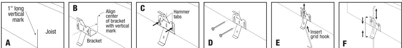
**IMPORTANT:** Do not cut QuickHang hooks. If the hook needs to be shortened due to an obstruction, the top portion can be bent by hand or with pliers.
