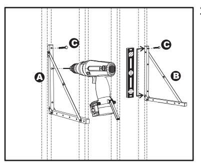
**1B:** Mount the Vertical Tubes of the Left & Right Brackets (A&B) with Lag Screws (C), using a 1/2" nut driver or socket wrench, making sure holes the are positioned as shown.
