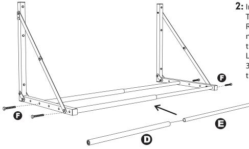
2: Insert the smaller diameter Round Tubes (E) into the larger diameter Round Tubes (D). Using a 9/16" nut driver or socket wrench, fasten them to the horizontal tubes of the Left & Right Brackets (A&B) with 3/8" x 2" Hex Bolts (F), in the position that best supports your tires.
