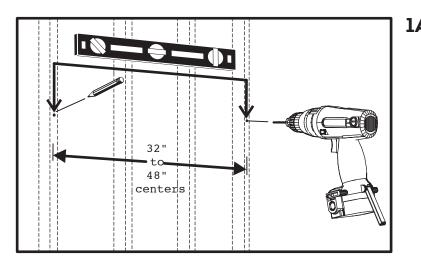
**1A:** Using a stud-finder, locate 2 wall studs that are 32" to 48" on center. Using a pencil, mark the top mounting hole centers. Make sure holes are level. Pre-drill the 2 marked holes using a 3/16" drill bit.
