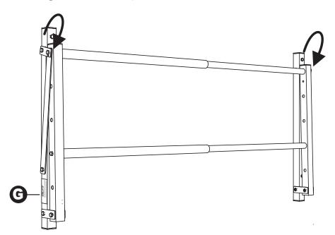
**3:** Make sure that all Fasteners are fully tightened and if necessary, adjust tightness so that the unit folds easily for storage. Store the unit in a folded position by locking it closed with the side hooks, as shown.
