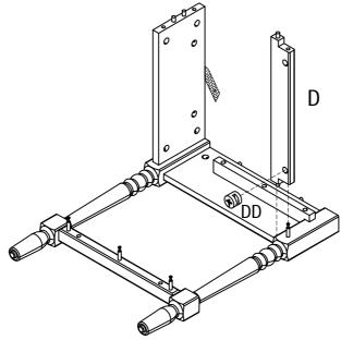
6 Connect bottom panel(F) with screw(DD) from step 5
