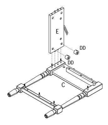
5 Connect front tie-bar panel(D) with cam lock(DD) from step 4
