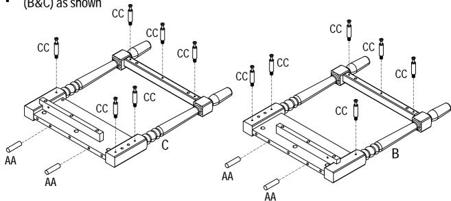
2 Locked cam bolt(CC) to drawer front panel(G) and table top panel(A) as shown
