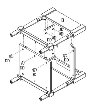
8 Connect table top panel(A) with cam lock(DD) from step 7
