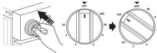
The electric spark ignition system makes a clicking noise.
