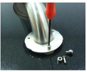
8. Attach bar to adapters using the screws & sleeves included. Make sure to re-attach in same position as originally set to be sure screws align properly. Tighten firmly. Slide cover ring over base and turn clockwise until properly aligned and turn to lock in place. Job complete!
