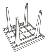
Repeat the same assembly process for the remaining three legs and respective screw points
