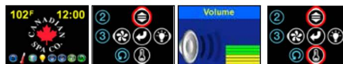
From the Home Screen, Touch the Audio Volume Button to open the Volume Control Menu. The Audio Volume Level Menu is Open, indicating the Volume Level.
