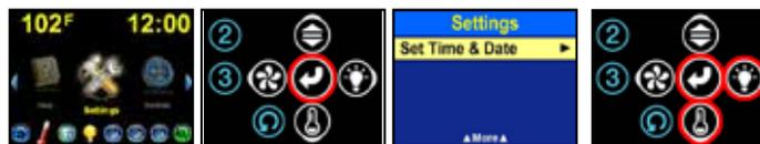
To Set Time & Date, in Navigation Mode, with Settings Highlighted, Touch Select to Open the Settings Menu. Scroll Down , and with Set Time & Date Highlighted, Touch Select or Right to Open the Set Time & Date Menu.
