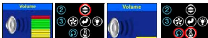
Touch the Up Button to Raise the Audio Volume Level, or Touch the Down Button to Lower the Audio Volume Level. Touch the Back Home Button to Exit the Volume Control Menu, or the Menu will Auto Exit in a few seconds.
