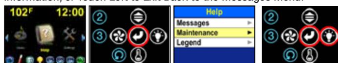
For Help with Maintenance, in Navigation Mode, Move Left or Right until Help is Highlighted, then Touch Select to Open the Help Menu. In the Help Menu, with Maintenance Highlighted, Touch Select or Right to Open the How To Menu.
