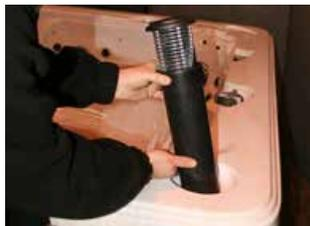
**STEP 5** - Screw in new speaker using body to tighten - removing nut and using fixed nut to spa until tight.
