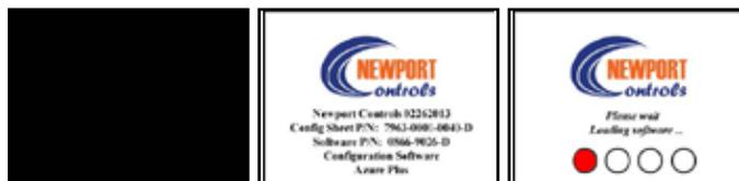
It will take 3 to 4 minutes for the Software to Load and Control System to Initialize. After the Power is ON, the Control Panel Backlighting will turn ON, but the Display Screen will remain Black for about 20 seconds. Then, for the next 20 seconds, there will be a Screen that shows the Serial and Part Numbers. At about 40 seconds after the Power is ON, there will be a Screen indicating that the Software is Loading.
