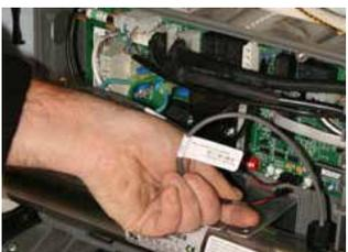
**STEP 5** - Unplug sensors plug from circuit board - Pinch tab down before pulling out plug.
