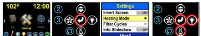
To Set the Heating Mode, in Navigation Mode, with Settings Highlighted, Touch Select to Open the Settings Menu. Scroll Down , and with Heating Mode Highlighted, Touch Select or Right to open the Heating Mode Menu.
