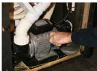
**STEP 7** - Unscrew earth wire from pump (ensure wire is moved safely away from pump area)
