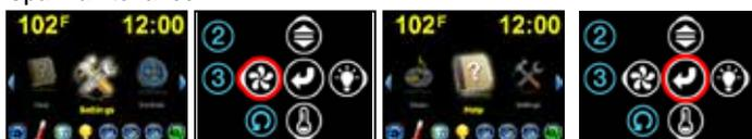
For Help with the Messages, in Navigation Mode, with Settings Highlighted, Move Left until Help is Highlighted, and then Touch Select to Open the Help Menu.
