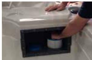
**Step 3.** Remove the old filter(s) by unscrewing them
