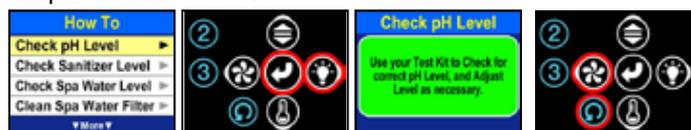
Scroll Up or Down to the desired Maintenance How To Menu Bar, and Touch Select or Right to View that Maintenance information. Then, Touch Left to Exit Back to the How To Menu. Touch Back Home to Exit back to the Home Screen.
