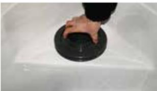
**Step 2.** To lift basket turn counter-clockwise until the flat part of the basket aligns with the flat part of the filter housing
