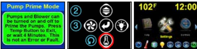
About 3-1/2 minutes after the power is turned ON, The Pump Prime Mode Screen will be displayed. At this time the Pumps can be manually turned On and Off. Pump Prime Mode will Auto Exit in about 4 minutes, or Press the Temp Button to Exit.
