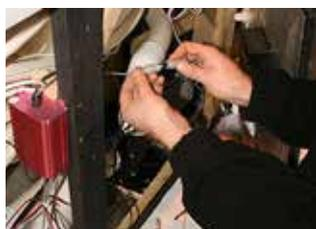
**STEP 2** - Unscrew nut and then unplug on/off connection from amplifier
