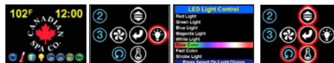
From the Home Screen, Touch the Light Button to open the LED Light Control Menu. On the Light Control Menu, Touch the Up and Down Buttons to Scroll to one of the Five LED Light Colors or one of the three LED Light Shows, then Touch Select to Change to that LED Light Control Option. Touch the Back Home Button to Exit the LED Light Control Menu, or the Menu will Auto Exit in a few seconds.
