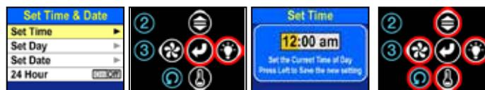
To Set the Time of Day, with Set Time Highlighted, Touch Select or Right to Open the Set Time Menu. To change the Time of Day, Move Right to Hours or Minutes, and then Touch Up or Down to change the Time. Touch Left to Save the new Time and Exit back to the Set Time & Date Menu, or Touch Back Home to Not Save the new Time and return to the Home Screen.
