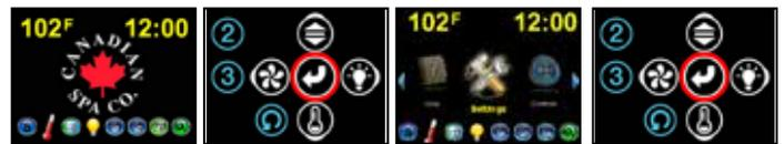
From the Home Screen, Touch the Select Button to change to Navigation Mode, with the Default Settings Highlighted. Touch the Select Button again to open the Settings Menu.
