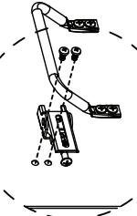
**Assemble lock as pictured using the 4 screws included**
