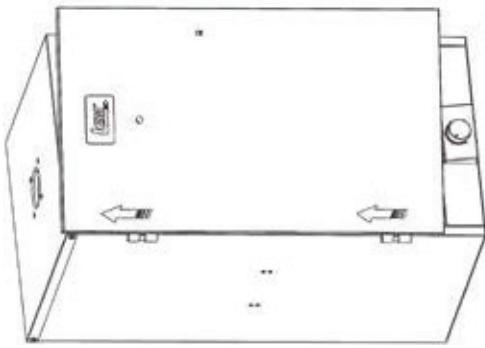
Door is easily removed by simply lifting straight up off the hinges.
