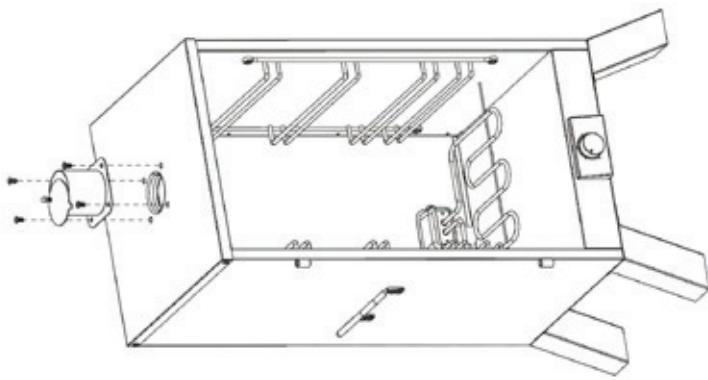
Assemble damper as pictured using the 4 screws included.
