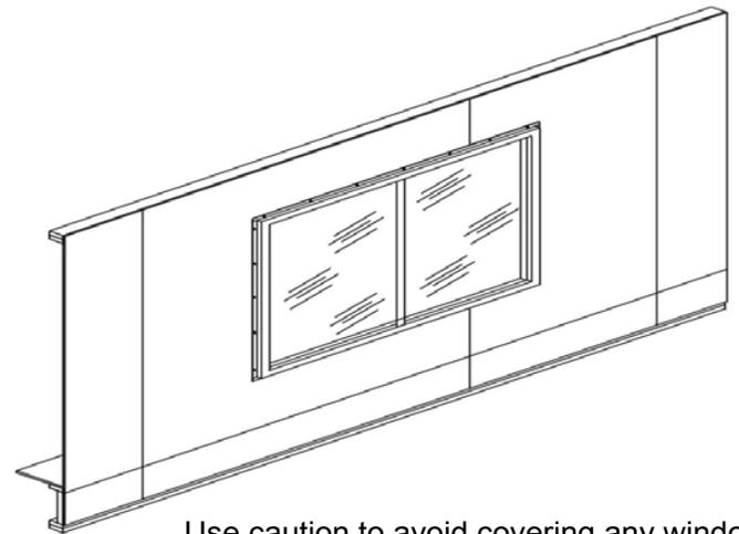
Use caution to avoid covering any window weep holes with sealant, paint or any other obstructive material
