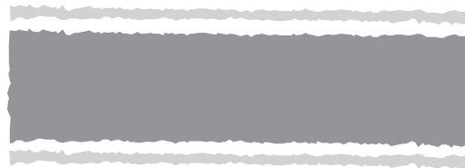
POOR SPRAY PATTERN (TAILING)
