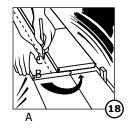
together lengthwise using a pull iron and a hammer. The cross-cut ends are tightened using a stop block or a pull iron and hammer.
