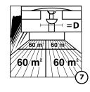
There should be an offset of at least 40 cm between the cross-cut ends of the floor panels in consecutive rows.
