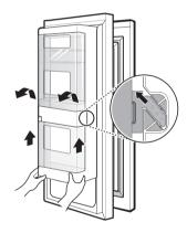
**2** Pull out the crisper to full extension, lift the front up, and pull straight out.
