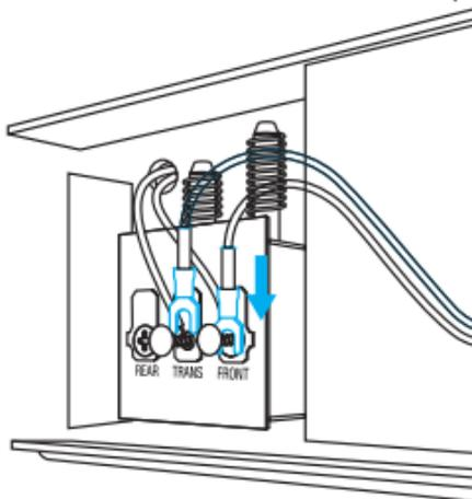
Locate the Chime Kit included in the smart doorbell's package and the terminals on the inside of the chime. Connect one of the Chime Kit's prongs to the transformer terminal (usually labeled TRANS, T, AC or 0). Connect the other prong to the chime's front terminal (usually labeled FRONT, F, 1 or C1). Either prong on the Chime Kit can be connected to either of the terminals on the chime.
