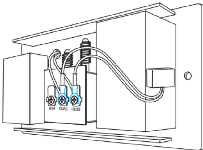
Ensure that the Chime Kit and wires DO NOT interfere with the mechanical parts of the chime. Mount on the outside of the chime if there is not enough room to mount inside and replace your chime's cover.
