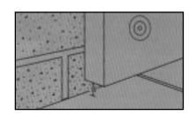
★ Insert the insulation panels into the J-Channels or set the foam tightly to the bottom of the siding if J-Channel is not used.
